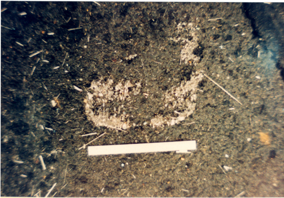
6. Cylinder Liner Fragment Impact with Asphalt Surface
